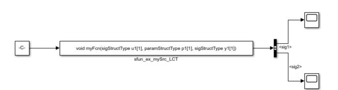
In the Constant block dialog box, the **Constant value** parameter is set to a structure whose fields match those of the structure type sigStructType. On the **Signal Attributes** tab, **Output data type** is set to the bus object sigStructType.
