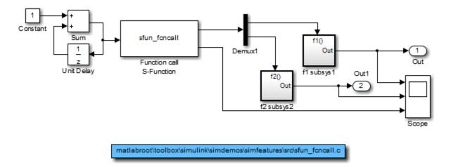
The first function-call subsystem provides a sine wave output. The second function-call subsystem is a simple feedback loop containing a Unit Delay block.
