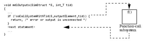
In this figure, ssCallSystemWithTid executes the function-call subsystem that is connected to the first output port element. ssCallSystemWithTid returns 0 if an error occurs while executing the function-call subsystem or if the output is unconnected. After the function-call subsystem executes, control is returned to your S-function.
